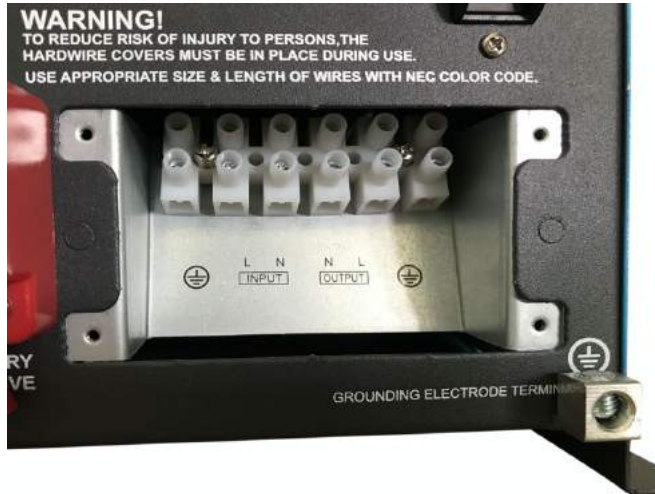
Figure 14 AC Wiring Compartment
